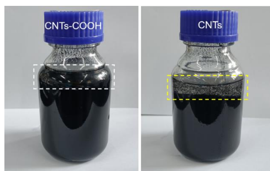
Fig. S2 Photo of CNTs with -COOH and unmodified CNTs dispersed in ethanol solution
