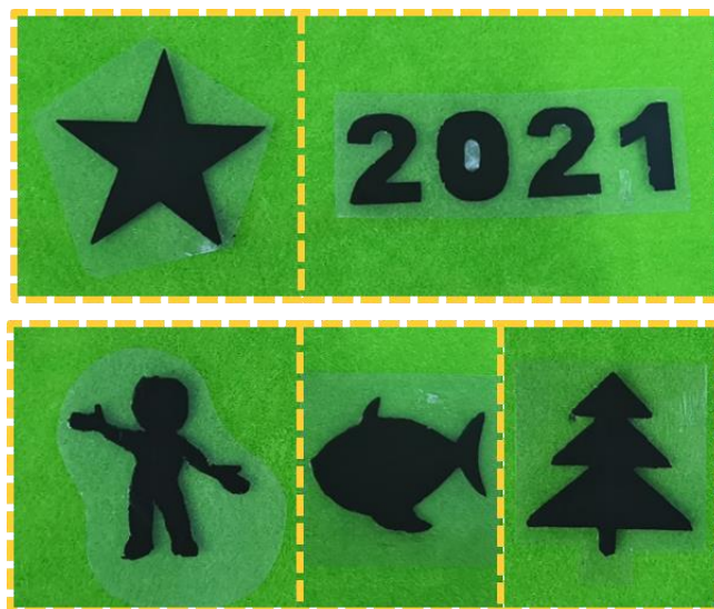
Fig. S20 Patterning of PCPM. PCPM was transferred to PET and then cut ted to get various patterns, including stars, numbers, small person, fish and trees.
