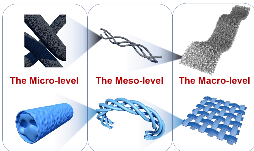
Fig. S6 The illustrations are used to explain the origin and essence of the flexibility of doped micro kink carbon nanofiber felt from the micro-, meso- and macro-levels
