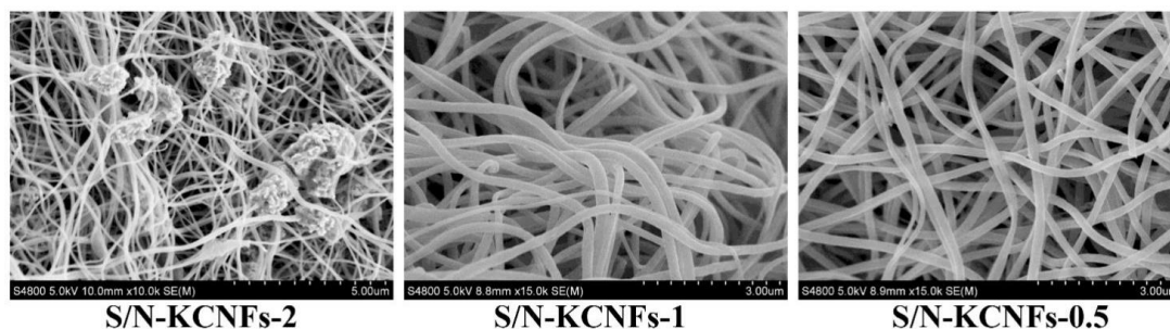
Fig. S10 SEM images of PAN: MA mass ratio in S/N-KCNFs were changed to 1:2 and 2:1
