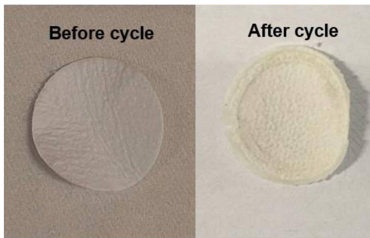
Fig. S9 Optical photos of separators disassembled SIC system after cycling for 100 cycles
