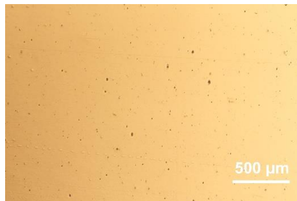
Fig. S10 Microscopic image of the tape surface after peeling off operation on the Janus film
