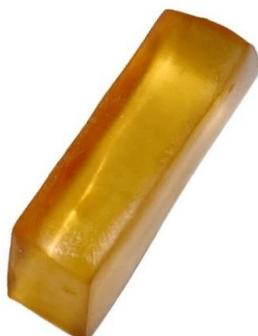
**Fig. S17** Photos showing the smooth surface of the 0.01 M-0.25 h PAAm/Fe-Alg hydrogel after cut
