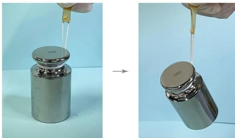
**Fig. S18** Photos showing the thin 0.01 M-0.25 h PAAm/Fe-Alg hydrogel lifting a 500-g weight
