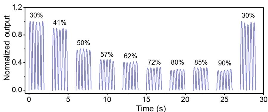
**Fig. S14** Durability test of the ITM under humidity conditions; Open-circuit voltage of the ITM under different humidity conditions
