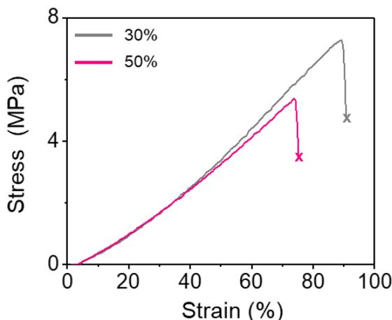
**Fig. S5** Stress-strain curve; Stress-strain curve of the ionic nanofiber electrodes with [EMI][TFSI] concentration of 30% and 50%
