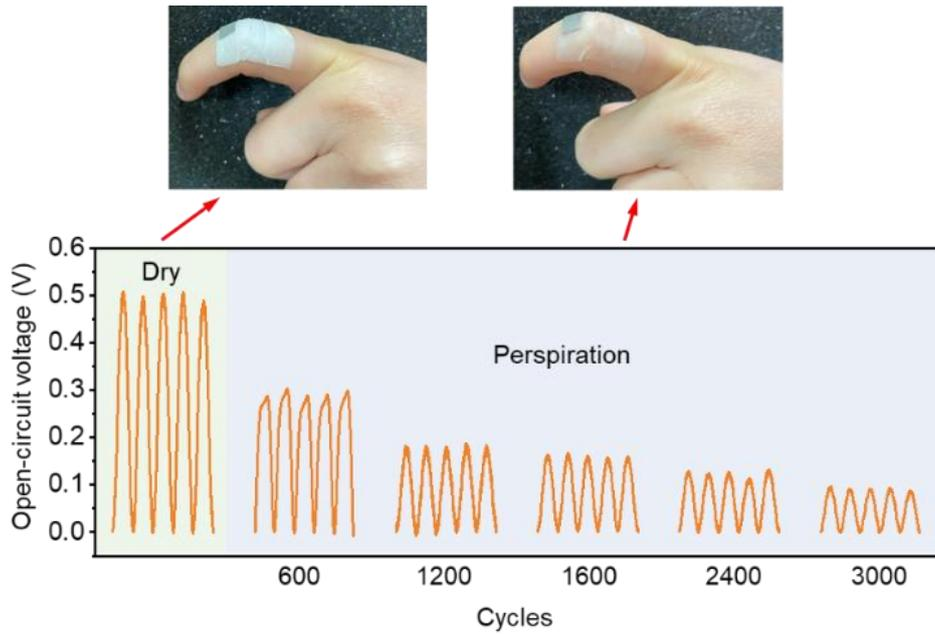
**Fig. S15** Durability test of the ITM under perspiration conditions; The photographs of the ITM attached on the finger joint under dry and perspiration conditions (top); Cyclic output tests of the ITM under sweating conditions (down)
