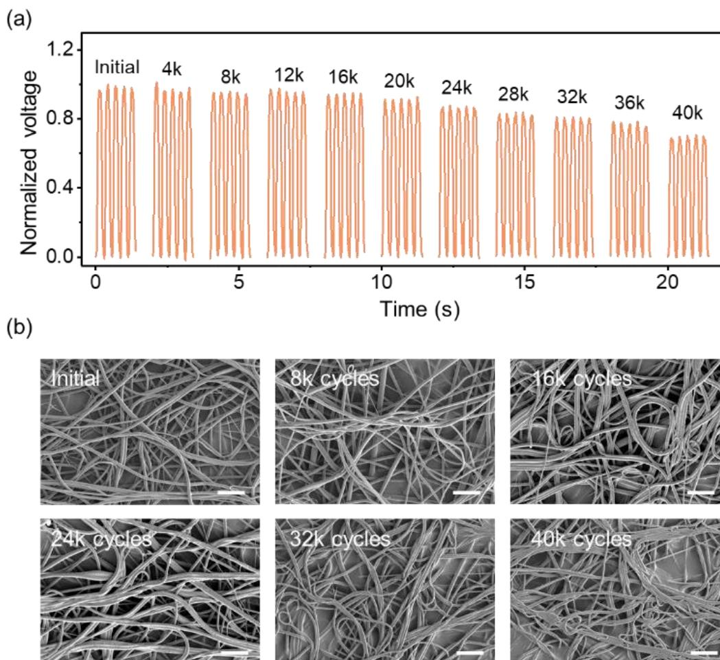
**Fig. S11** Durability test of the ITM after sliding for 40000 cycles; **a** Open-circuit voltage of the ITM after sliding for 30000 cycles; **b** SEM images of the ITM surface after sliding cyclic test (Scar bar is 10 μm)
