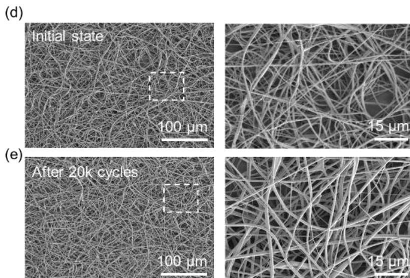
**Fig. S13** Durability test of the ITM after stretching for 20000 cycles; **a** Open-circuit voltage of the ITM after stretching for 20,000 cycles; **b** SEM images of the ITM surface after stretching cyclic test
