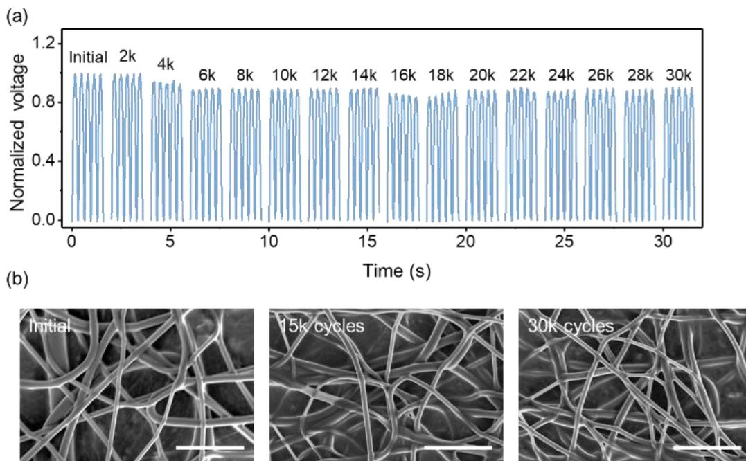
**Fig. S12** Durability test of the ITM after bending for 30000 cycles; **a** Open-circuit voltage of the ITM after bending for 30000 cycles; **b** SEM images of the ITM surface after bending cyclic test (Scar bar is 10 μm)
