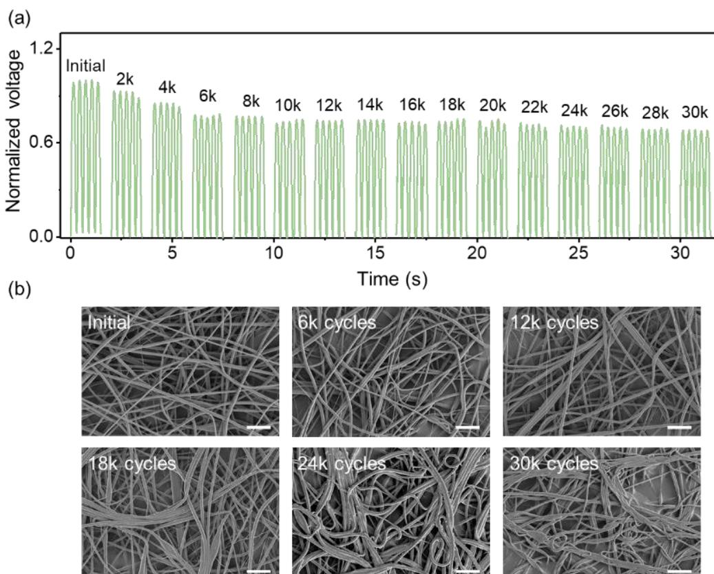
**Fig. S10** Durability test of the ITM after contacting for 30000 cycles; **a** Open-circuit voltage of the ITM after contact-separation for 30000 cycles; **b** SEM images of the ITM surface after contact-separation cycles (Scar bar is 10  $\mu\text{m}$ )
