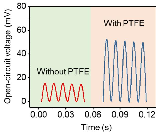
**Fig. S18** Open-circuit voltage measured from the ITM with and without the PTFE film (with SPL of 55.7 dB and frequency of 110 Hz)
