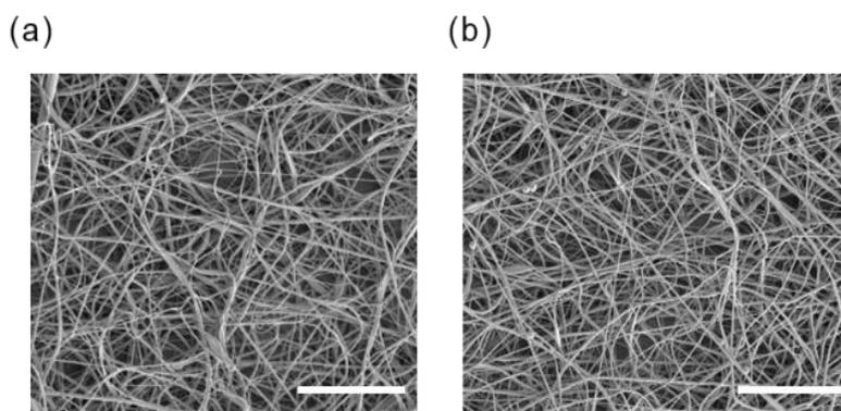
**Fig. S7** SEM characterization of the surface morphology of the ITM; **a** SEM images for the initial surface morphology for the ITM; **b** SEM images for the ITM surface after being stretched over 20000 cycles (Scar bar is 50  $\mu\text{m}$ )
