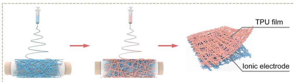
**Fig. S1** The fabrication procedures of the ITM through electrostatic spinning process; The ITM is fabricated by two-step electrospinning technology; (i) The electrospinning process of the ionic electrode layer; (ii) The electrospinning process of the TPU layer. The TPU nanofibers were electrospun directly on the above electrode layer
