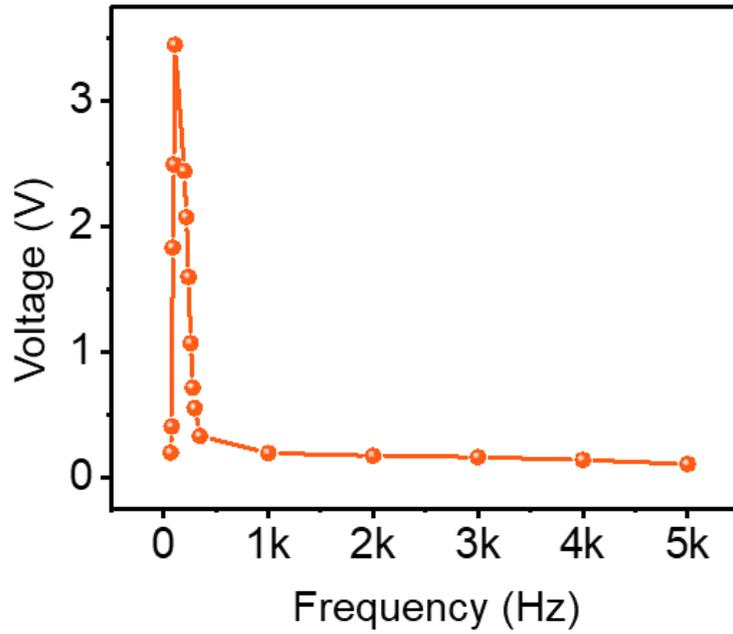
**Fig. S19** Typical voltage signal of the ITM under the variable acoustic frequency; The relationship between open-circuit voltage of the ITM and the sound frequency (sweeping frequency ranges from 70 to 5000 Hz; sound intensity is 87.3 dB SPL)
