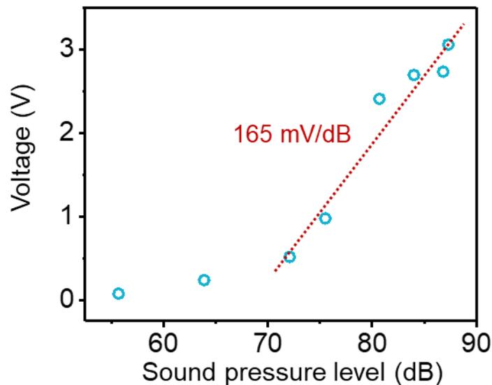
**Fig. S16** Sensitivity of the ITM for acoustic energy sensing; The relationship between open-circuit voltage of the ITM and the sound pressure level (SPL)
