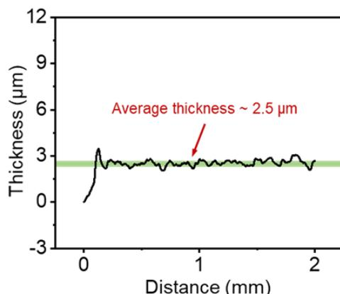
**Fig. S2** Thickness characterization of the ITM; The thickness of the ITM membrane measured by the step profiler; The roughness of the surface is attribute to three-dimensional hierarchical stacked nanofiber networks
