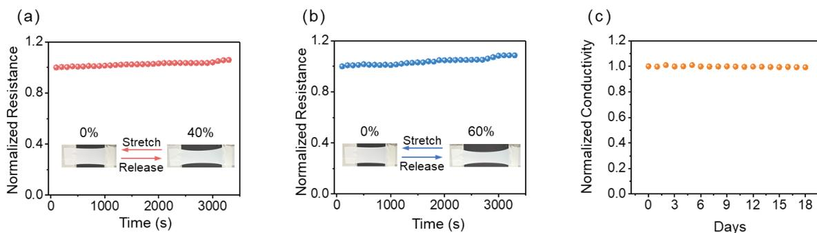
**Fig. S6** Cyclic performance of the ionic electrode; **a** The relative resistance variations of the ionic electrode against cyclic strain at 40%; **b** The relative resistance variations of the ionic electrode against cyclic strain at 60%; **c** Conductivity variations of the ionic electrode after storage for three weeks at room temperature
