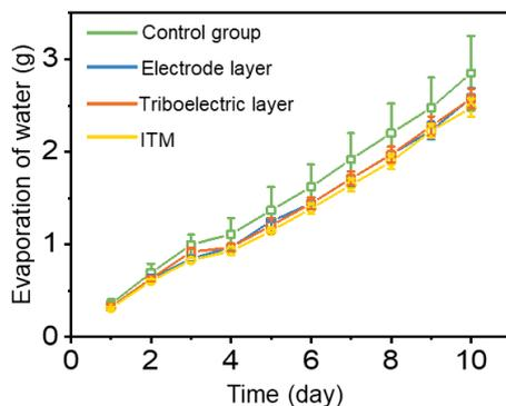
**Fig. S3** Permeability property of the ITM; Water vapor permeability property of the pure TPU triboelectrification layer, ionic nanofibers electrode and the ITM membrane
