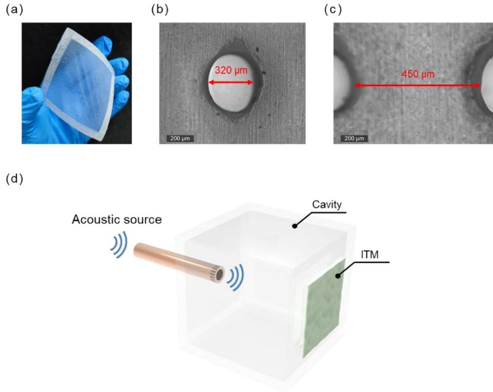
**Fig. S17** Acoustic testing by the ITM; **a** Photograph of the PTFE film with acoustic holes distributed. (Scale bar: 1 cm); **b** Optical microscope photograph of the acoustic holes; **c** The gap between the acoustic holes; **d** Structure scheme of the Helmholtz resonant cavity for harvesting acoustic energy
