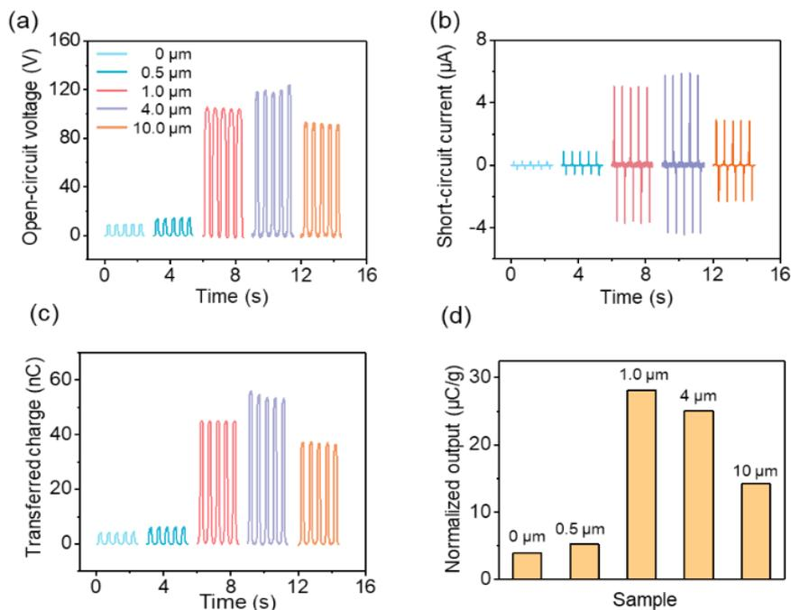
**Fig. S8** The output performance of the ITM when the TPU triboelectrification layer was fixed at 2  $\mu\text{m}$ ; **a** Open-circuit voltage; **b** Short-circuit current; **c** Transferred charges and **d** Normalized output of the ITM when varying the thickness of the ionic electrode
