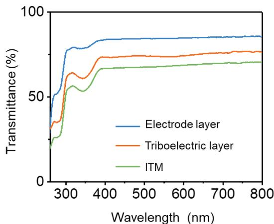
**Fig. S4** Optical transmittance characterization; Optical transmittance spectra for the pure TPU triboelectrification layer, ionic nanofibers electrode and the ITM membrane
