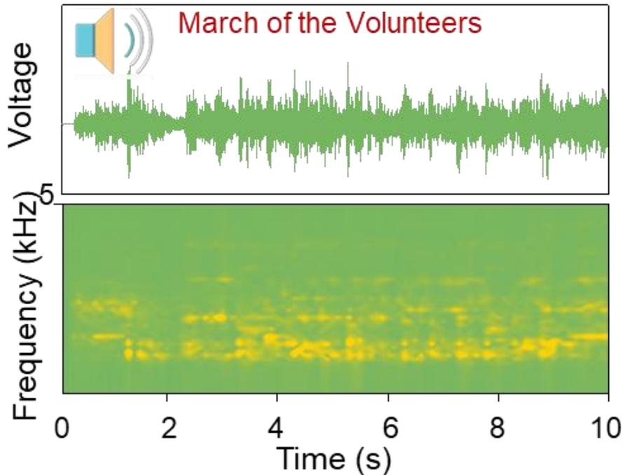
**Fig. S20** Waveform and frequency spectrogram signals of melody “March of the Volunteers” extracted by the ITM; Real-time voltages capture and display of the decoded frequency-domain information
