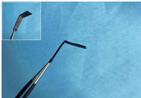
Fig. S7 Digital image of GO/HCPA paper after being burned, it still can be bent beyond 90°, showing a certain extent of structural stability
