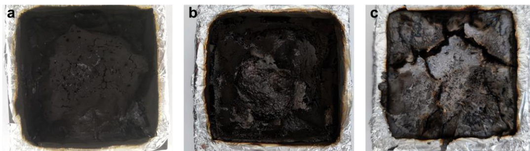
Fig. S24 Digital photos of residue chars for a pure RPU foam b FRPU-2.0 and c FRPU-4.0
