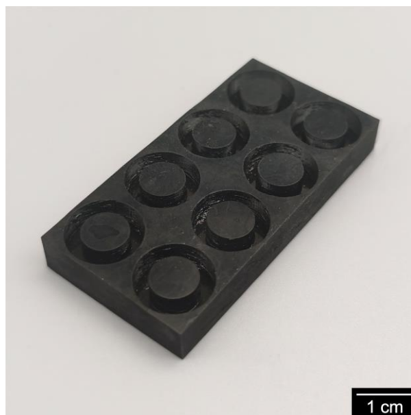
Fig. S11 Si–O–C ceramic metamaterial structure fabricated for EM wave absorption in X–Ku band
