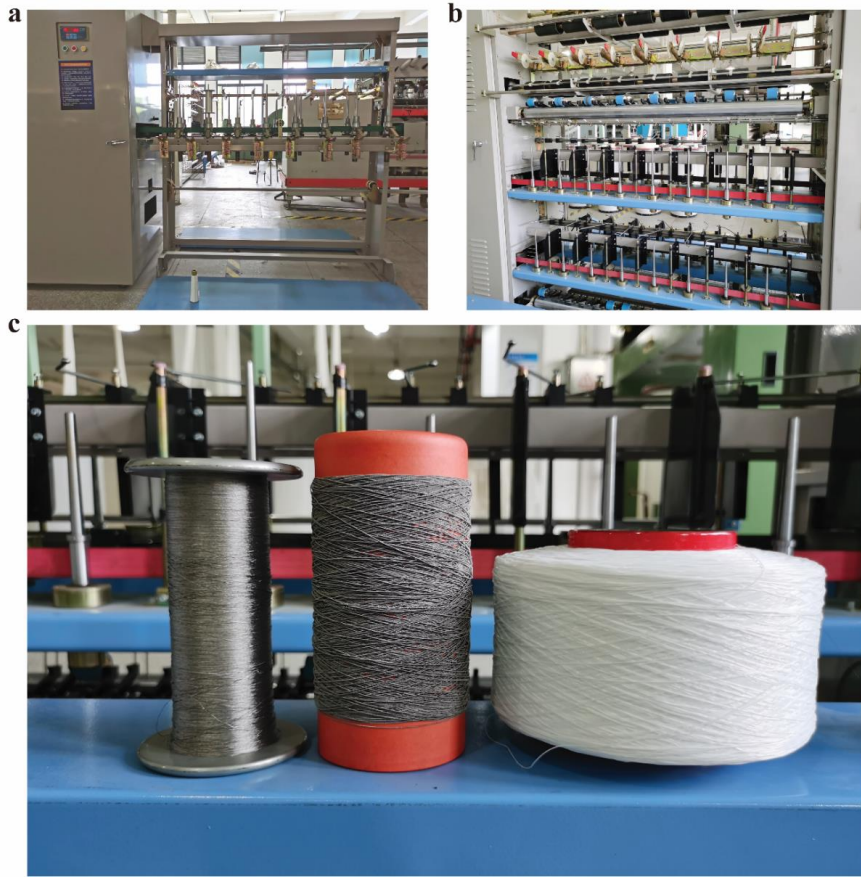
Fig. S2 Pictures showing the continuous and mass-producible AIYS spinning technology. (a) Yarn pressing machine, which is used to prepare the bobbin of wrapping yarn. (b) Hollow spindle twister machine for fabricating the AIYS. (c) Pictures show the core yarn (right), sheath yarn (left), and AIYS yarn (middle)
