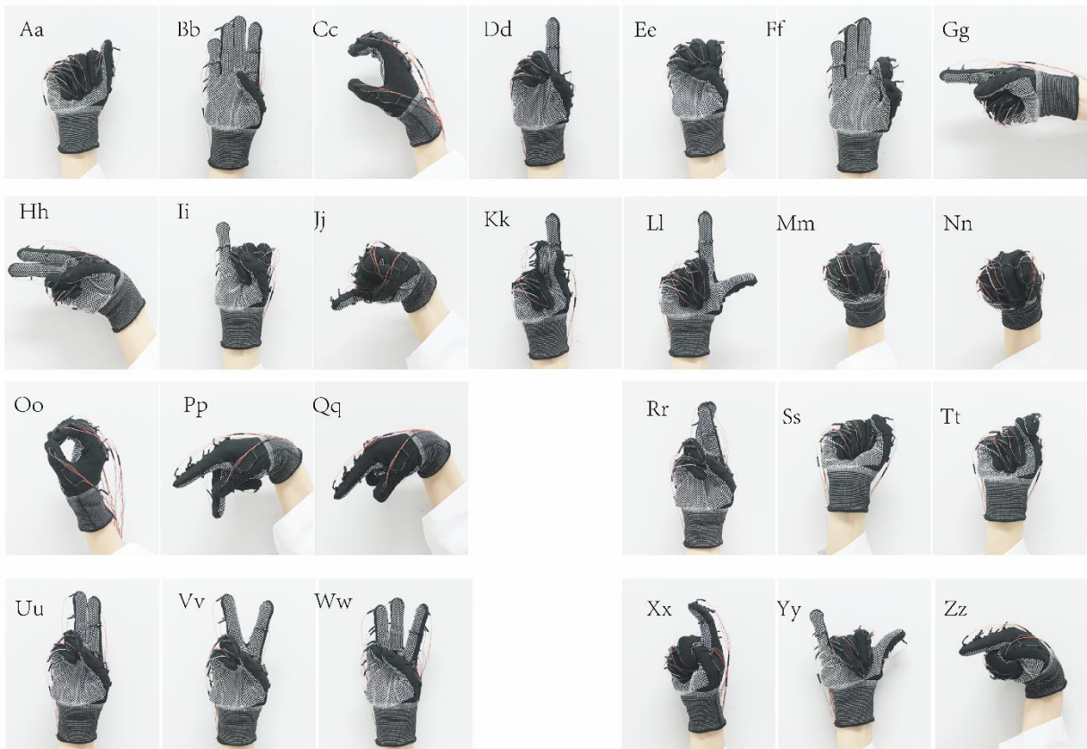
Fig. S14 Pictures showing the sign-language gestures of 26 letters of the English alphabet made by the volunteer according to ASL when wearing the smart glove with 16 AIYSs
