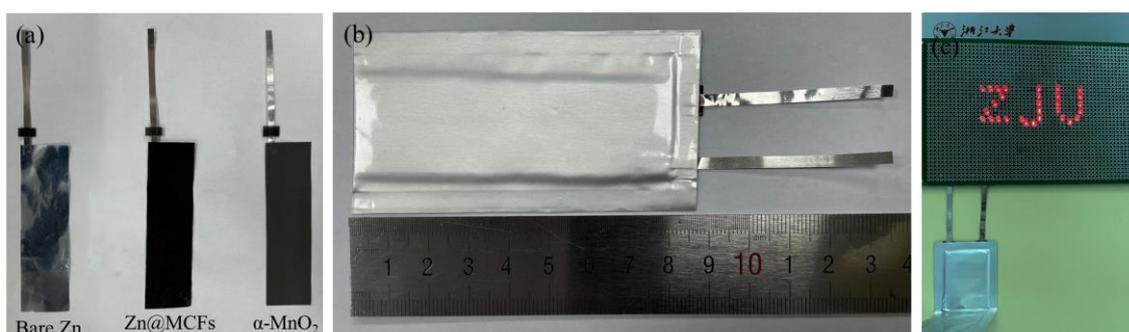
**Fig. S37** Optical photographs of (a) bare Zn, Zn@MCFs, and  $\alpha$ -MnO<sub>2</sub> electrodes, (b) pouch battery with Zn@MCFs anode and  $\alpha$ -MnO<sub>2</sub> cathode (size: 2×8 cm<sup>2</sup>), (c) digital photograph of 30 LEDs lit by the bent (90°) Zn@MCFs|| $\alpha$ -MnO<sub>2</sub> pouch battery
