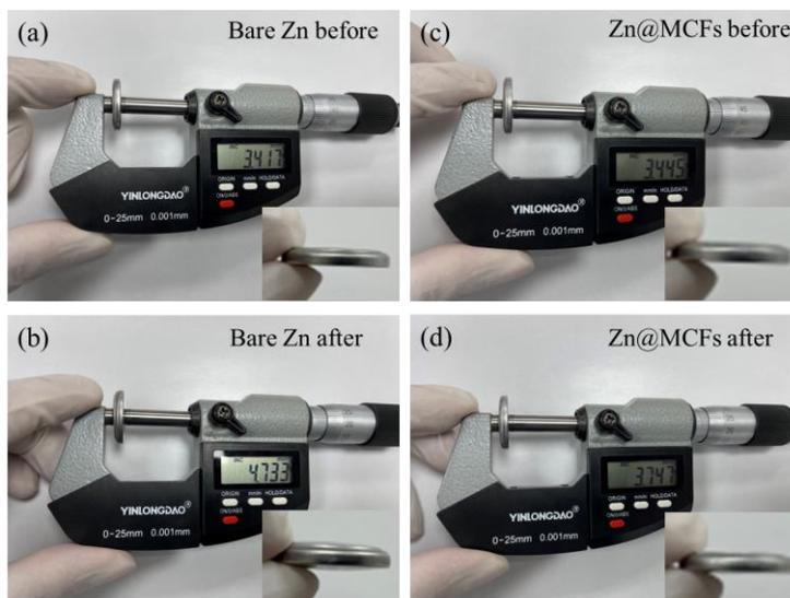
**Fig. S20** Thickness of (a,b) bare Zn and (c,d) Zn@MCFs symmetric cells before and after plating/stripping test ( $1 \text{ mA cm}^{-2}$ )
