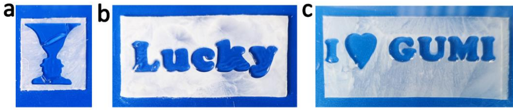
Fig. S7 Patterned crystallized touch-responsive smart hydrogel with various patterns, including (a) pattern of “cup”, (b) English word of “Lucky” and (c) the phrase of “I ♥ GUMI”
