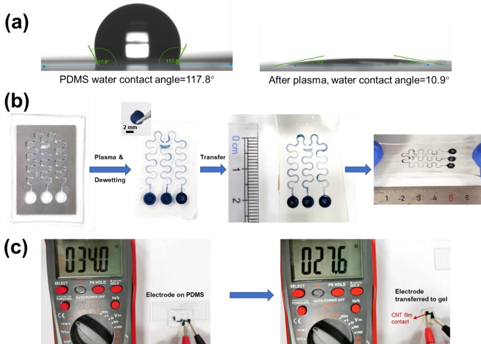
Fig. S4 a Contact angle measurements of hydrophobic PDMS substrate before and after oxygen plasma treatment. b Fabrication process of patterned hydrophilic and hydrophobic PDMS surface using oxygen plasma under a stainless steel mask to form the PEDOT:PSS/LiTFSI patterns on PDMS by dewetting, followed by transfer printing to obtain stretchable microelectrodes on the gel substrate. c Resistance values of the PEDOT:PSS/LiTFSI electrode before (left) and after (right) transfer onto GEL-GLY/ \text{Na}_3\text{Cit} . The soft carbon nanotube (CNT) thin films were used for contact pads
