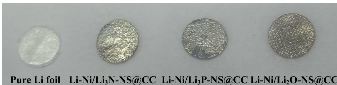
Fig. S8 The digital photos of pure Li foil, Li-Ni/Li 3 N-NS@CC, Li-Ni/Li 3 P-NS@CC, and Li-Ni/Li 2 O-NS@CC
