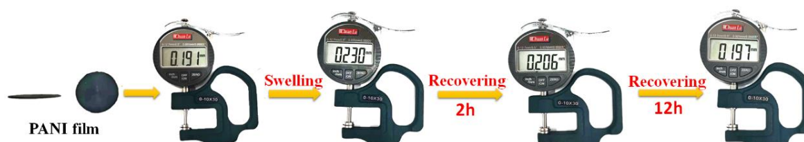
Fig. S14 The swelling experiment and the thickness changing of PANI were measured using a digital thickness gauge
