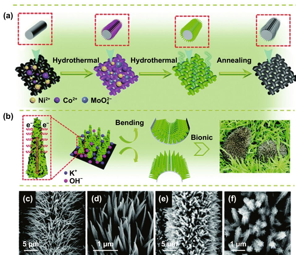
Fig. 5 a Schematic illustrations of \text{NiCo}_2\text{O}_4@ \text{Ni}_x\text{Co}_y\text{MoO}_4 nanostructures (carbon fabric (black), \text{NiCo}_2\text{O}_4 nanoneedle clusters (pink), the \text{NiCo}_2\text{O}_4@ \text{Ni}_x\text{Co}_y\text{MoO}_4 precursor (green), \text{NiCo}_2\text{O}_4@ \text{Ni}_x\text{Co}_y\text{MoO}_4 (gray)); b charge transport and stress release in these hedgehog-like nanoneedle-cluster nanostructures; c , d SEM images of \text{NiCo}_2\text{O}_4 nanoneedle clusters; and e , f \text{NiCo}_2\text{O}_4@ \text{Ni}_x\text{Co}_y\text{MoO}_4 nanostructures. Reproduced with permission from Ref. [119]. Copyright 2018, Royal Society of Chemistry
