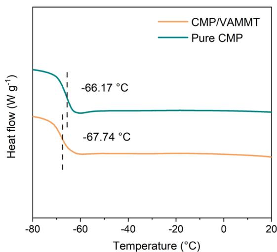
**Fig. S8** DSC curves of CMP/VAMMT and pure CMP
