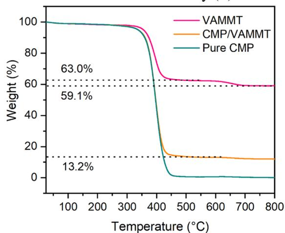
**Fig. S11** TGA curves of CMP/VAMMT and pure CMP
