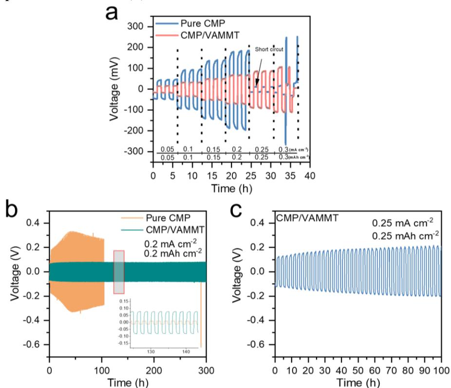
**Fig. S14** Critical current density tests on CMP/VAMMT and Pure CMP in symmetric cell, each cell was cycled three times at specific current density (a). Long-term cycling of symmetrical Li/Li cells with CMP/VAMMT and pure CMP at 0.2  $\text{mA cm}^{-2}$ , the lithium plating capacity is 0.2  $\text{mAh cm}^{-2}$  per cycle (b). The cycle performance of Li/CMP/VAMMT/Li at critical current density (0.25  $\text{mA cm}^{-2}$ , 0.25  $\text{mAh cm}^{-2}$ ) (c)
