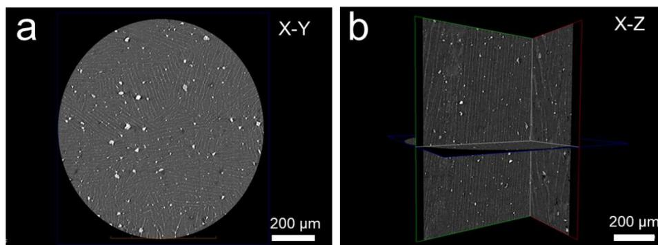
**Fig. S9** the internal sectional images of VAMMT in the X-Y plane (a) and X-Z plane (b) exhibit vertical array-like structure of VAMMT
