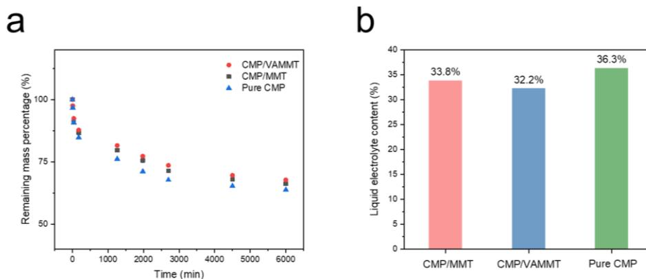
**Fig. S12** Changes in the quality of different GPEs over time in an oven at 80°C (a). Content of liquid electrolyte in different GPEs (b)
