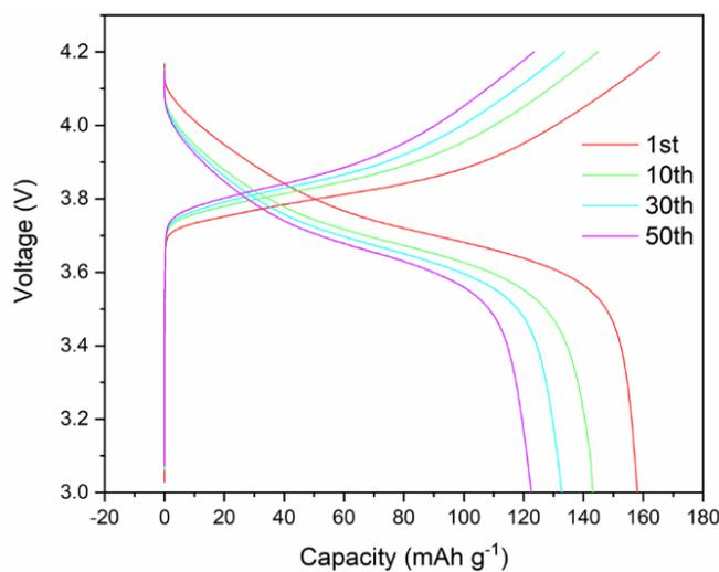
**Fig. S25** Corresponding voltage profile of Li/CMP/VAMMT/NCM523 cell at the 1, 10, 20, 40 cycles
