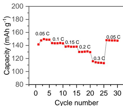
**Fig. S20** Rate performance of Li/CMP/VAMMT/LFP at 0 °C
