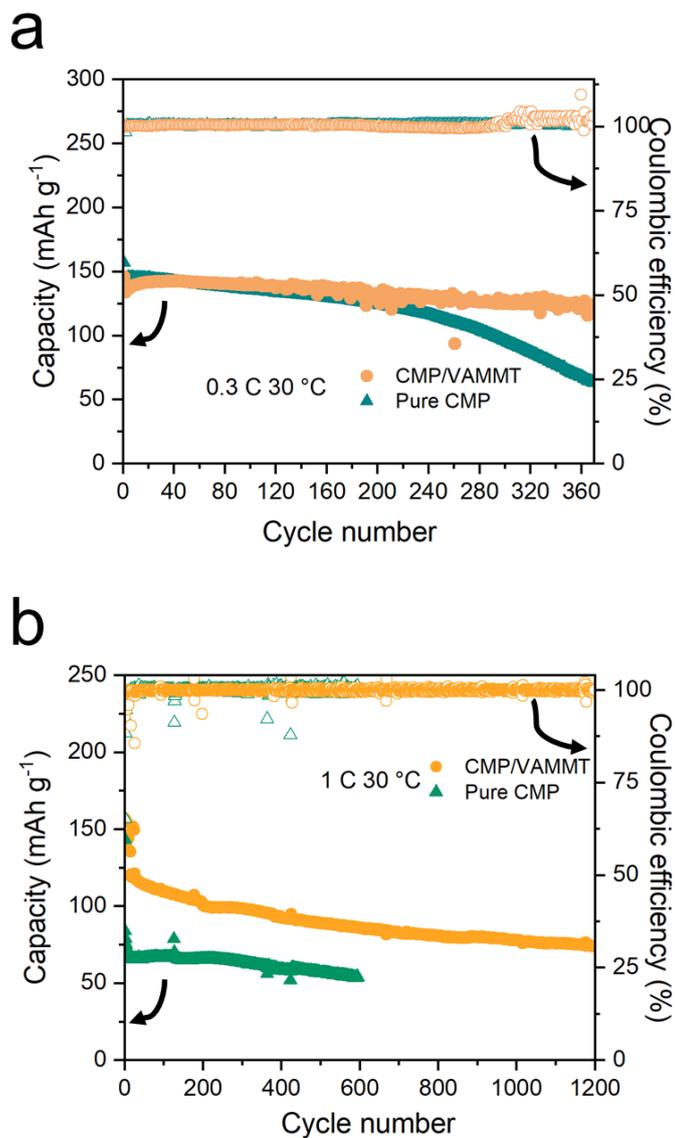
**Fig. S22** Long cycle performance of CMP/VAMMT and pure CMP at 0.3 C, 30°C (a); 1 C, 30°C (b) in the Li/LFP cells
