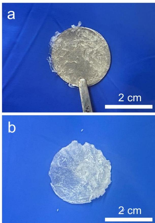
**Fig. S16** Optical photo of Pure CMP with Li anode (**a**) and CMP/VAMMT membrane (**b**) in symmetrical Li cells after the 20th cycle (corresponding to Fig. 4g-h)
