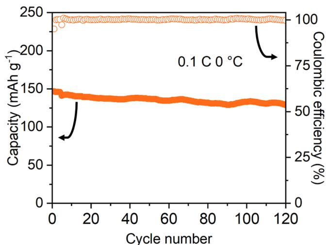
**Fig. S21** Long cycle performance of CMP/VAMMT at 0.1 C, 0°C in the Li/LFP cells
