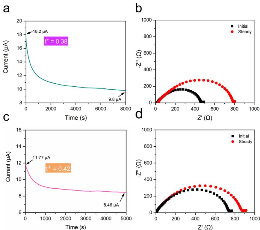
**Fig. S13** Current variation with time during polarization of Li/CMP/MMT/Li (a) with the initial and steady-state AC impedance (b) and Li/Pure CMP/Li (c) with the initial and steady-state AC impedance of the cell (d)
