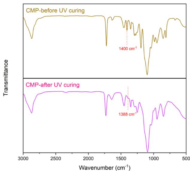
**Fig. S6** The Fourier transform infrared (FT-IR) transmittance spectra of CMP before (top) and after (bottom) UV curing
