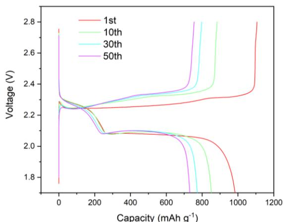
**Fig. S26** Corresponding voltage profile of Li/CMP/VAMMT/S cell at the 1, 10, 30, 50 cycles
