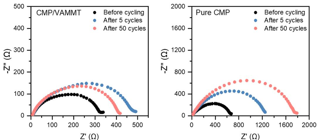
**Fig. S15** The EIS Nyquist plots of Li/GPE/Li symmetrical cells
