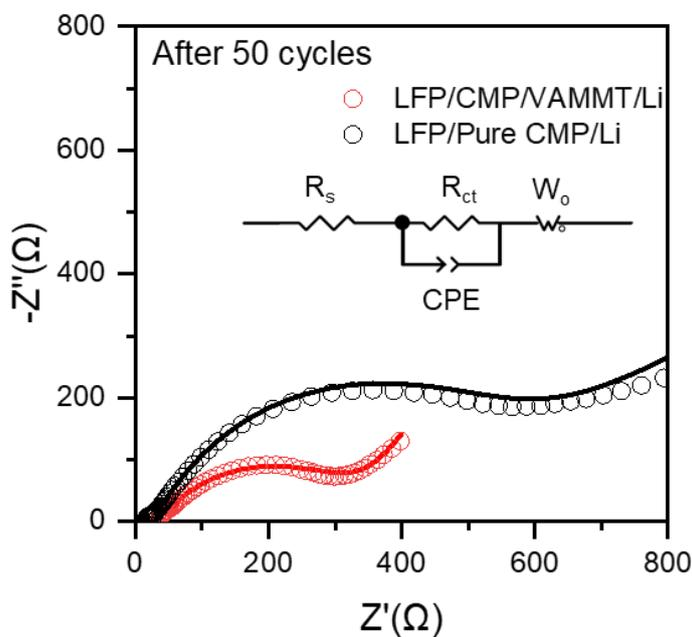
**Fig. S24** EIS curve of LFP/CMP/VAMMT/Li and LFP/pure CMP/Li cells after 50 cycles at 0.5 C, 30°C
