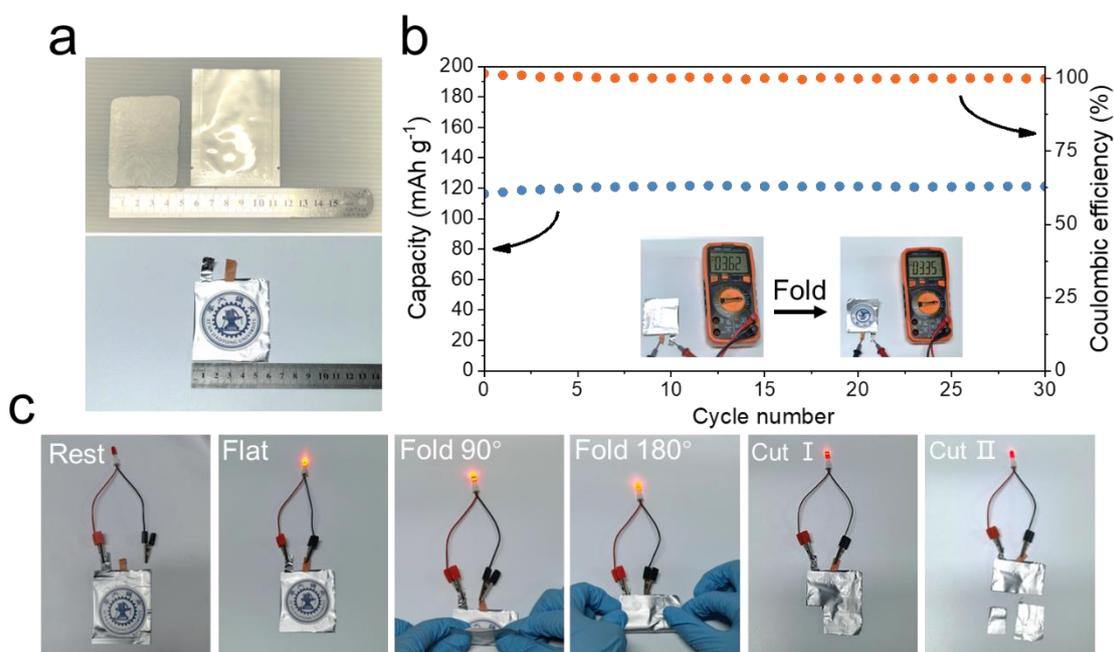
**Fig. S27** Digital photo of larger size VAMMT (above) and Li//LFP pouch cell with CMP/VAMMT (bottom) (a). Cycle performance of LFP/CMP/VAMMT/Li pouch cell at 0.2 C, 30°C (b). optical images of folding and cutting test of pouch-type LFP/CMP/VAMMT/Li cell (c)
