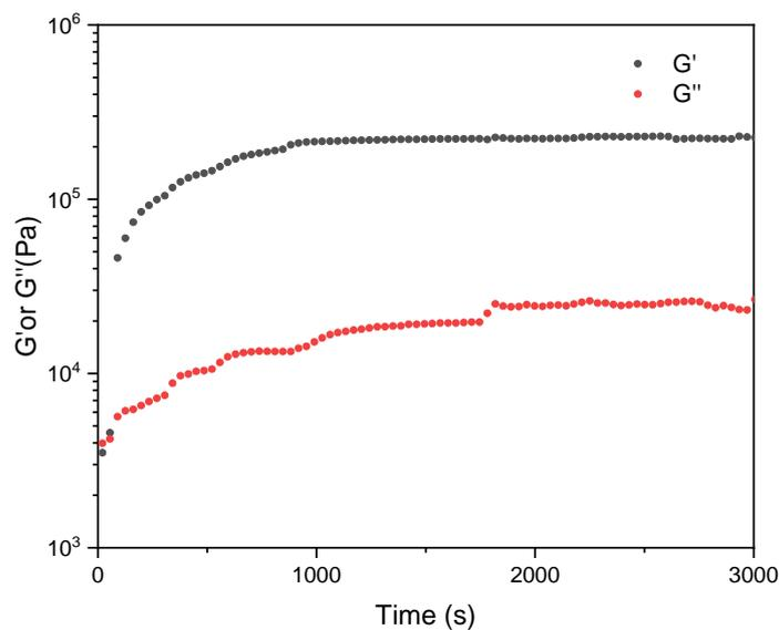
**Fig. S4** Variation of storage modulus ( $G'$ ) and loss modulus ( $G''$ ) with polymerization time
