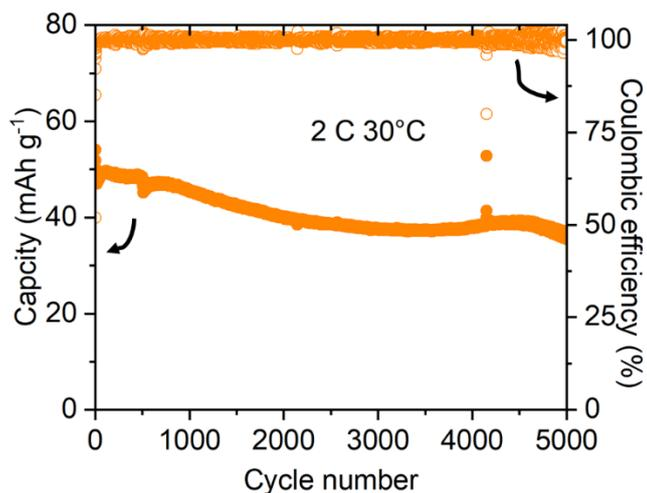
**Fig. S23** Long cycle performance of CMP/VAMMT at 2 C, 30°C in the Li/LFP cells
