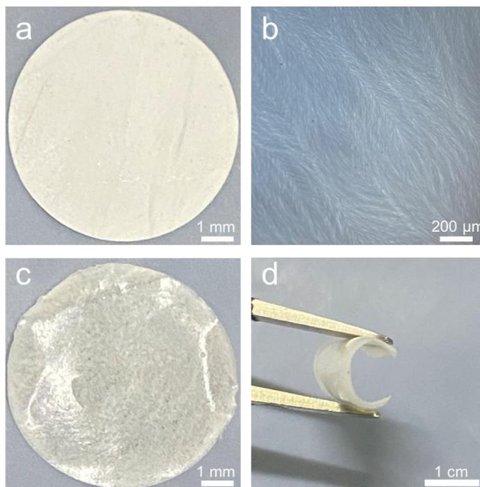
**Fig. S10** Digital image of small-size VAMMT (a) with an optical image (b) and small-size CMP/VAMMT (c) with a demonstration of the flexibility (d)
