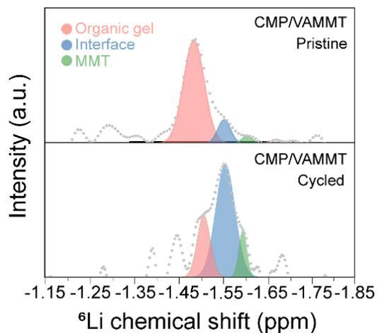
**Fig. S17** The  ${}^6\text{Li}$  SSNMR spectra of CMP/VAMMT before and after cycling in the  ${}^7\text{Li}\|\text{Cu}$  cell
