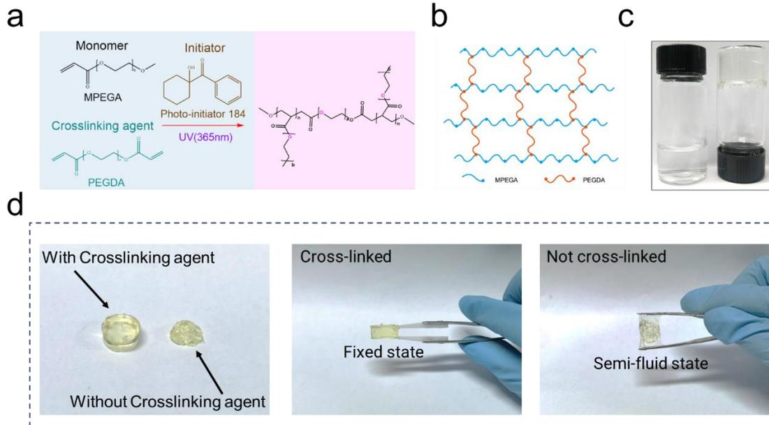
**Fig. S3** The cross-linking process of gel polymer (a) with schematic diagram (b). The digital photo of liquid precursor(left) and gel polymer(right) (c). Comparison of digital photos of gel polymer before and after adding crosslinking agent (d)
