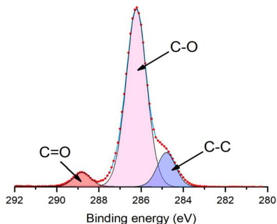
**Fig. S7** C 1s X-ray photoelectron spectroscopy (XPS) spectrum of CMP after UV. The absence of the C=C peak after curing indicates successful polymerization
