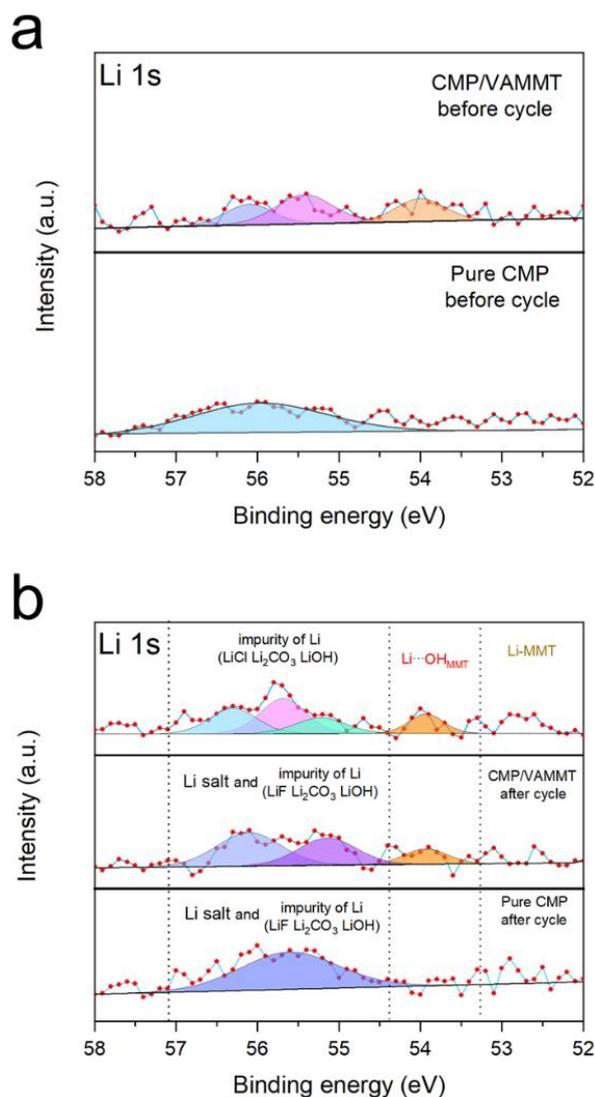
**Fig. S18** Li 1S X-ray photoelectron spectroscopy (XPS) spectra of CMP and CMP/VAMMT before (a) and after (b) cycling
