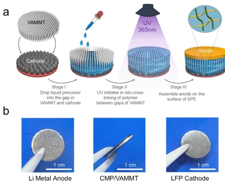
**Fig. S19** Schematic diagram of the full cell assembly process (a) and digital photos of the LFP cell with CMP/VAMMT (b)
