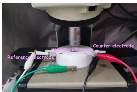
Fig. S29 Digital photograph of the chemical cell for using in in-situ Raman measurement
