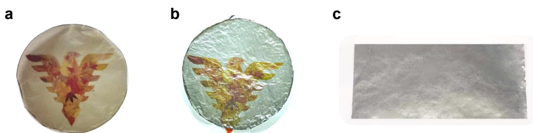
Figure S4. 50 nm-thick nMAG with a round shape before (a) and after (b) 3000 °C heat treatment. (c) 600 nm-thick nMAG with a rectangle shape after 3000 °C heat treatment.
