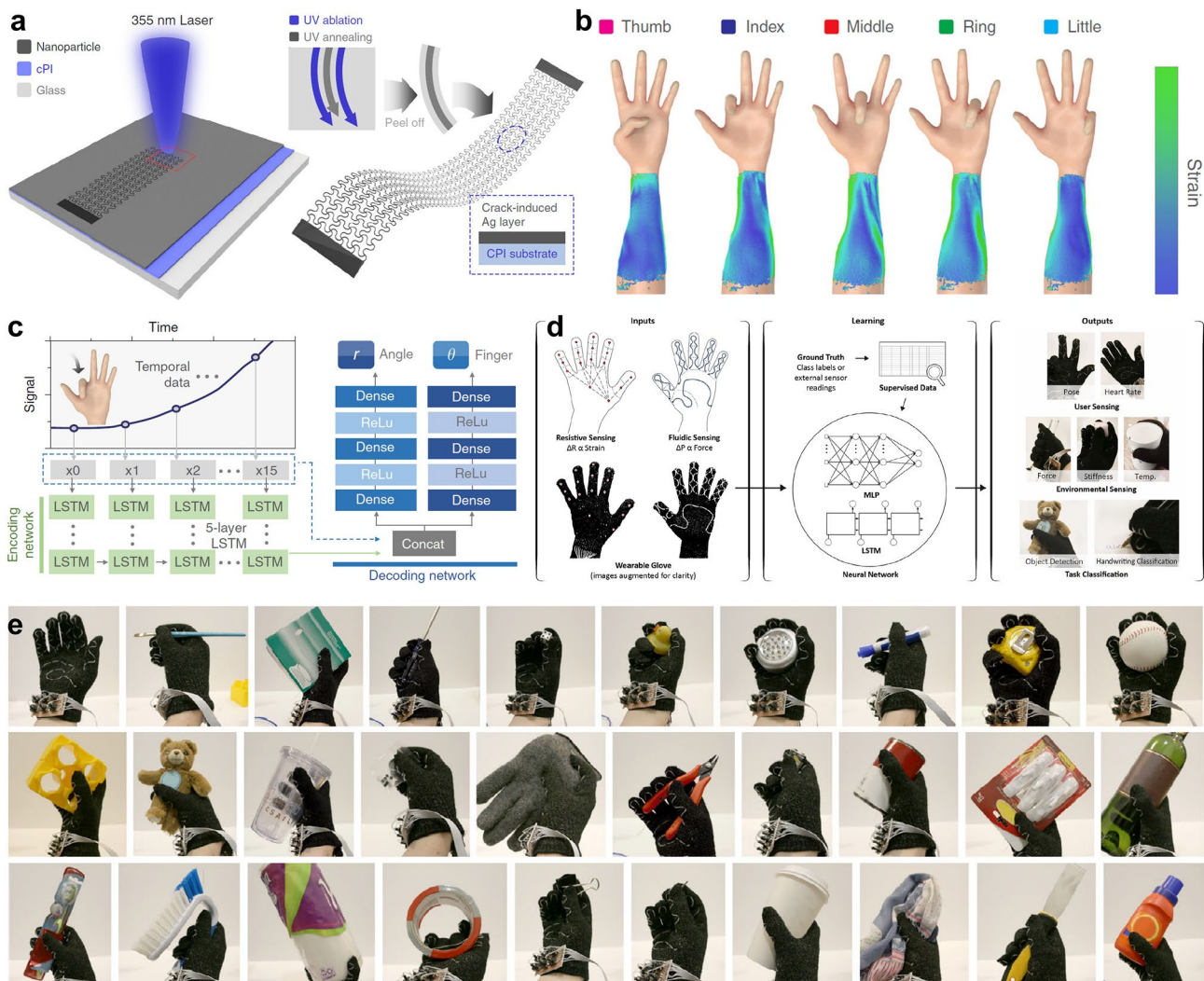
Fig. 29 RNN for the classification task. a Schematic depicting the patterning and crack fabrication by laser fabrication. b Depiction of skin deformations for different finger bending motions. c Neural network composed of an encoding network and a decoding network. LSTM layers are used in encoding network to analyze temporal sensor patterns to generate latent vectors. Two independent dense layers map created latent vectors to the metric space expressing hand motions. Dropout is used as the regularization technique to prevent the network to be overfitted to a single use case. Reproduced with permission [344]. Copyright (2020), Springer Nature. d Resistive sensing and fluidic sensing are combined to provide signals for strain and contact force information, respectively. These signals are fed into a pretrained neural network architecture for inference, which is trained from captured data labeled with ground-truth knowledge. Depending on the neural network, the output of the network provides inference for a wide variety of downstream tasks. Electrode points which are usually not visible have been colored and enlarged in the left-hand images for clarity. e Object classification dataset, with associated grasps. Reproduced with permission [34]. Copyright (2020), Wiley-VCH
