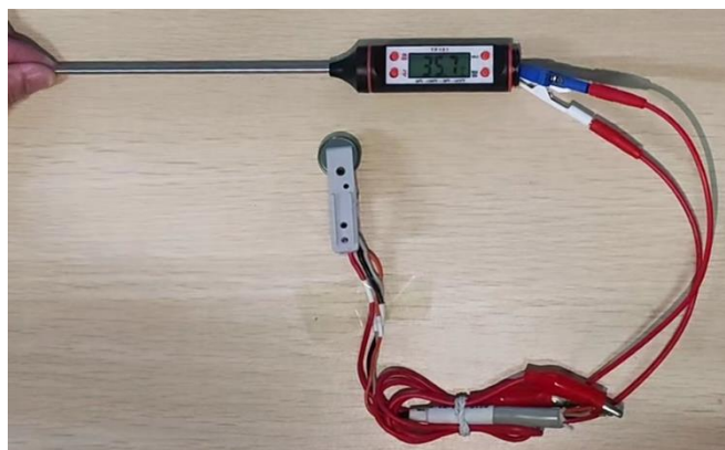
Fig. S8 Digital photos of the VGs-Li 2 S/LiPON/Pre-Li cell (sealed with CR2025-type coin cell) connected with a small thermometer
