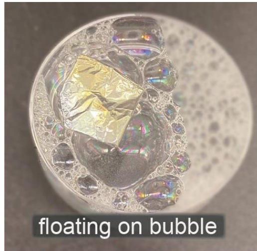
Fig. S3 The freestanding BCZT thin film with supporting layer EVA and bottom electrode Pt floats on water bubbles
