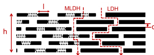
Scheme S1 Mass transfer path of MLDH and LDH membrane
