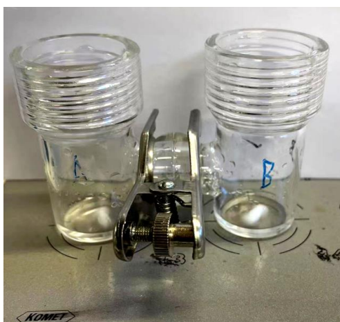
Fig. S12 A self-made U-shaped device to investigate the ion permeation behavior
