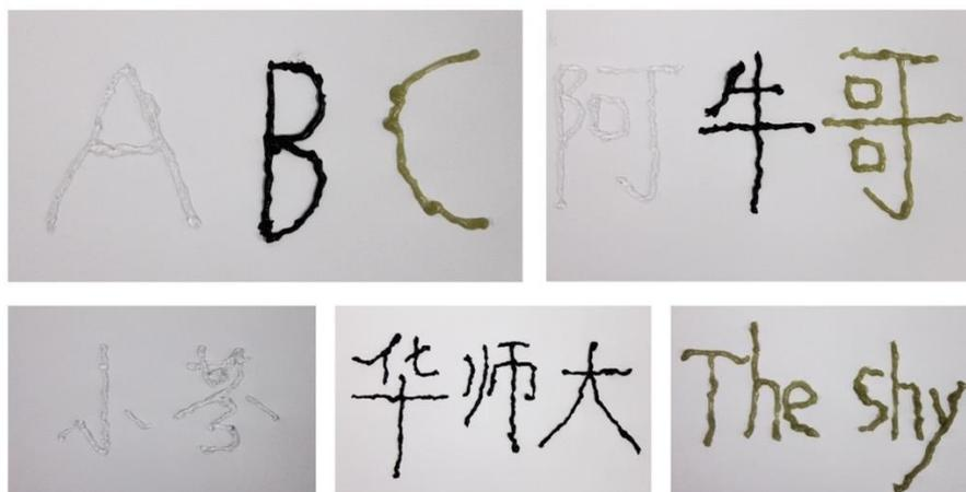
**Fig. S4** The injectability of NSFSG (white), CINPs@NSFG (black), and AgNWs@NSFG (yellow) through the syringe
