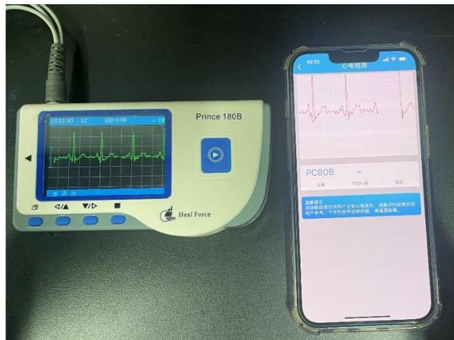
**Fig. S21** Photograph showing the wireless ECG recorder and the dynamic heart rate graph displayed on the APP
