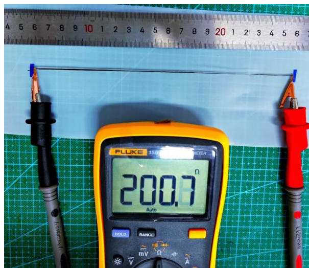
Fig. S2 The optical images of the resistance test of the CNT ribbon. The 20 cm-CNT ribbon has a resistance of 200.7 \Omega . The line resistance of the CNT ribbon is about 10 \Omega \text{ cm}^{-1}
