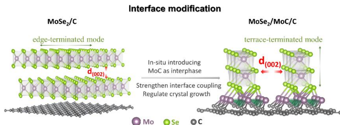
Scheme S1 Schematic illustration of models of MoSe 2 /C and MoSe 2 /MoC/C heterostructure
