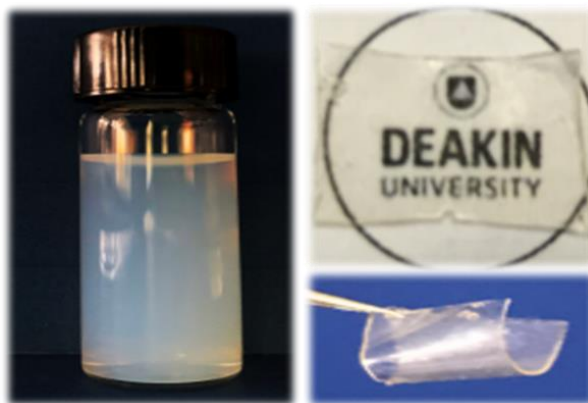
Fig. S7 The optical pictures of the W-SPU water dispersion and the as-obtained transparent W-SPU membranes
