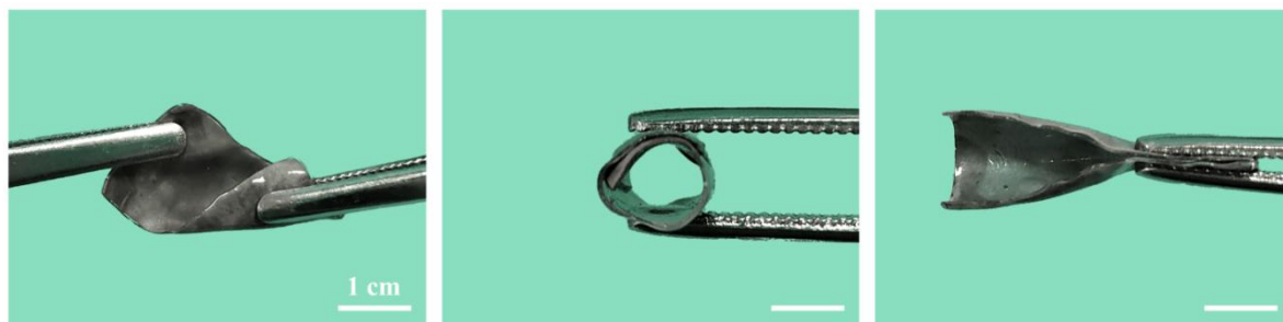
Fig. S7 Images of twisting, rolling and folding the composite organohydrogels, demonstrating the flexibility of the materials
