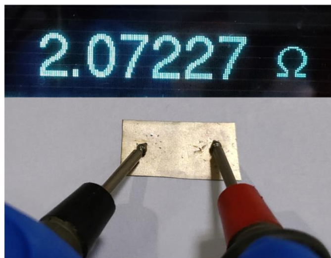
Fig. S4 The photograph of the PVP/Ag@PU nanofiber composite membrane with an ultralow resistance
