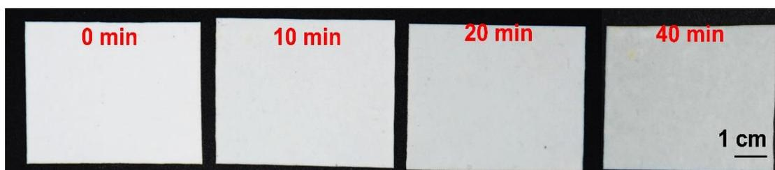
**Fig. S6** Digital photos of tSPM fabrics treated for different times under 150 °C
