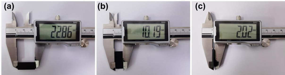
Fig. S14 The digital photographs of ov\text{-Nb}_2\text{O}_5/\text{CNS} -cyanate plate with a size of 22.9 mm×10.2 mm×2 mm
