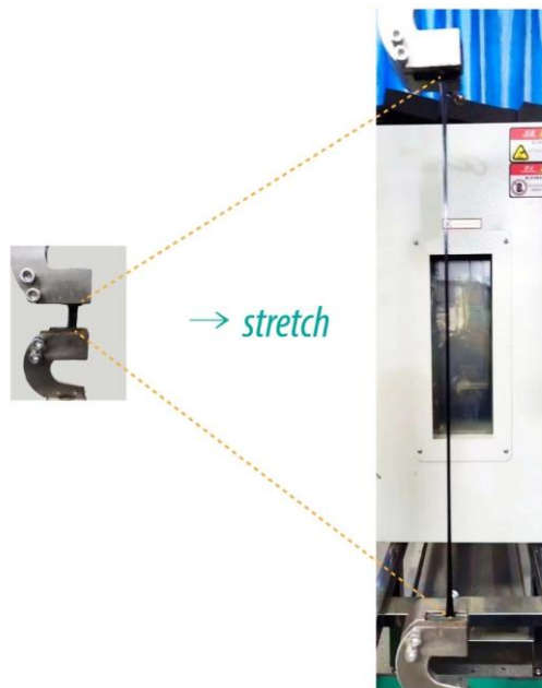
Fig. S5 Optical images showing the high stretchability of the PAA-MXene/HCF-GdmCl hydrogel
