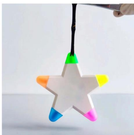
Fig. S8 An optical image showing using the PAA-MXene/HCF-GdmCl hydrogel to hang a plastic object after self-healing
