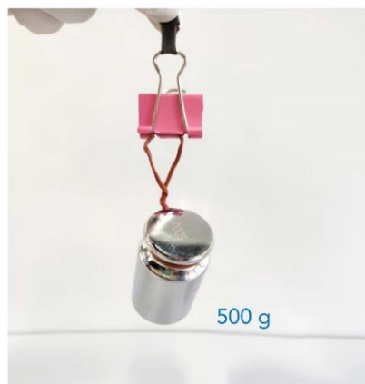
Fig. S6 An optical image showing using the PAA-MXene/HCF-GdmCl hydrogel to hang a 500 g weight
