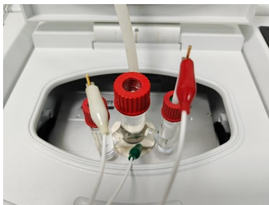
Fig. S19 The electrochemical cell for in situ ATR-FTIR measurement
