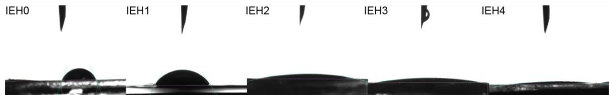
Fig. S13 Water contact angles of IEHs in the same testing time
