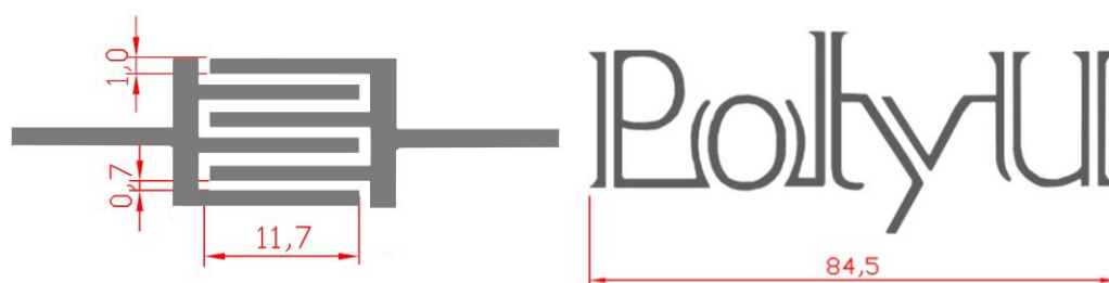
Fig. S1 The predesigned specifications and dimensions of the in-plane SCs in mm
