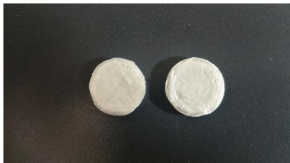
Fig. S15 Digital photographs of the separators of Na 0.95 LNCFM electrode after 50 cycles
