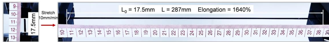
Fig. S5 Conductive polymers with 20% graphene content have great tensile properties, using a tensile tester to stretch the sample at 10 mm/min, showing 1640% tensile properties
