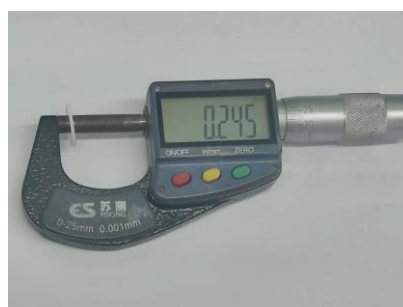
Fig. S6 The thickness of the PHL composite layer with various mass ratio of 1:3
