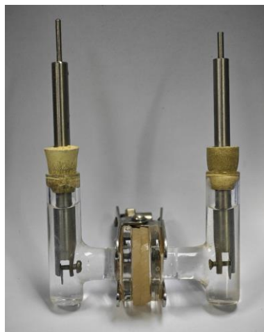
Fig. S14 Symmetrical cells assembled in transparent H-type tanks
