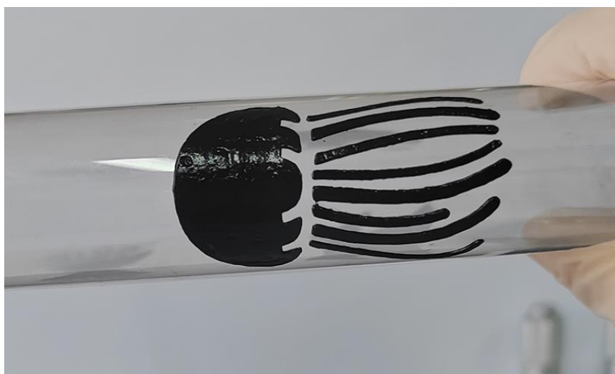
Fig. S27 Photograph of the jellyfish-shaped MXene gel coating on a PET substrate in the bending state
