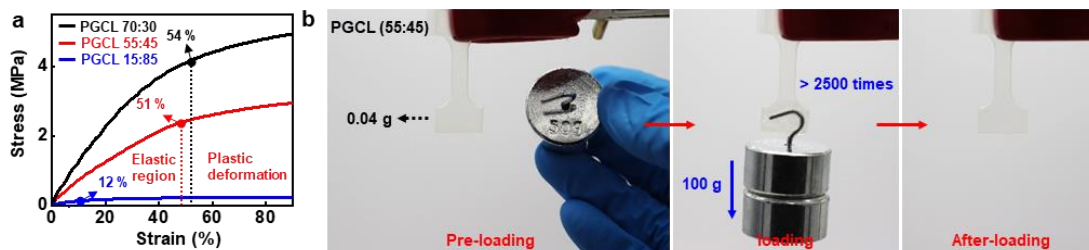
Fig. S5 Resilience and toughness of PGCL film. a Strain-stress curve in the initial condition of different PGCLs. b Toughness test images of PGCL (55:45) film loading with 100 g weights
