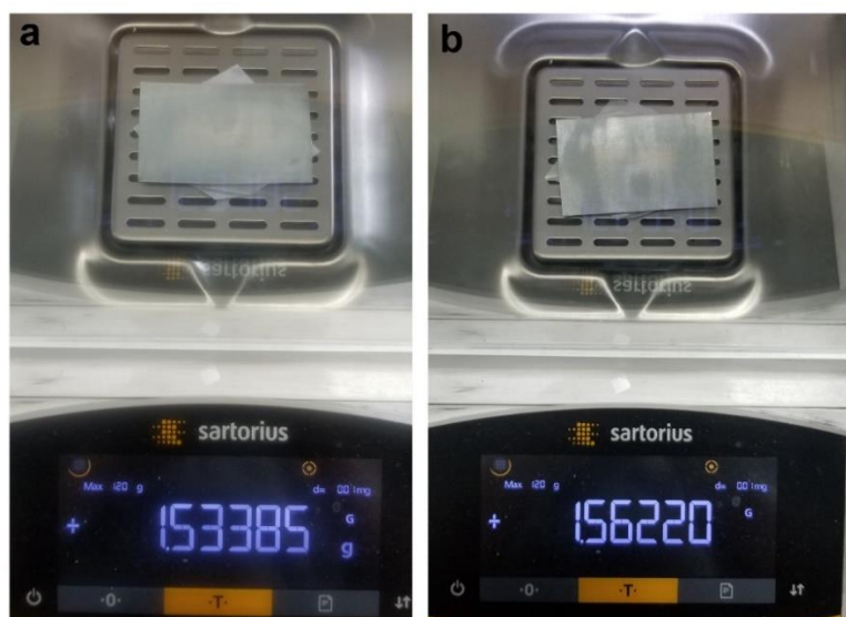
Fig. S3 Optical photographic image of the P-Zn electrode before and after In powder modification
