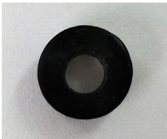
Fig. S1 The coaxial ring of materials with paraffin matrix for measurement of electromagnetic parameters and microwave absorbing performances
