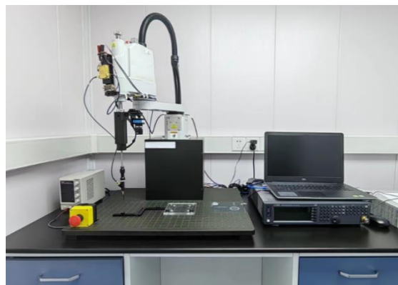
Fig. S10 Measuring equipment of near-field shielding performance
