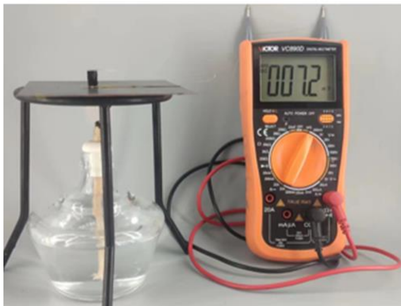
Fig. S7 Photograph showing the generated voltage of the aerogel sensor by harvesting alcohol lamp flame heat energy
