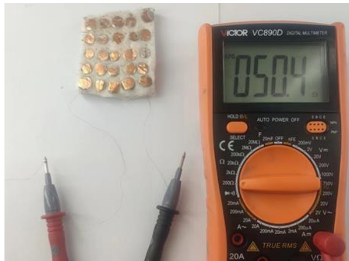
Fig. S11 The internal resistance of the aerogel-based TE generator
