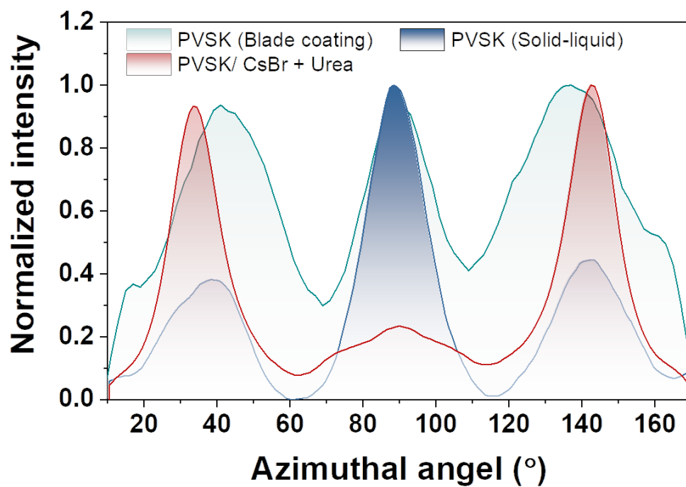
Fig. S5. Normalized integrated intensities of the perovskite (100) planes as marked in Fig. 3a-3c and plotted as a function of the azimuthal angle.
