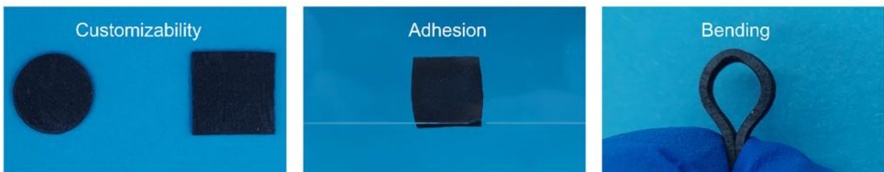
Fig. S1 The fabricated composite film is easily customizable, self-adhesive, and bendable
