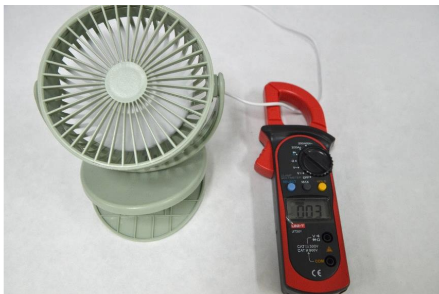
Fig. S9 Alternating current of 3A and 50 Hz AC generated by a fan to simulate the external electromagnetic interference
