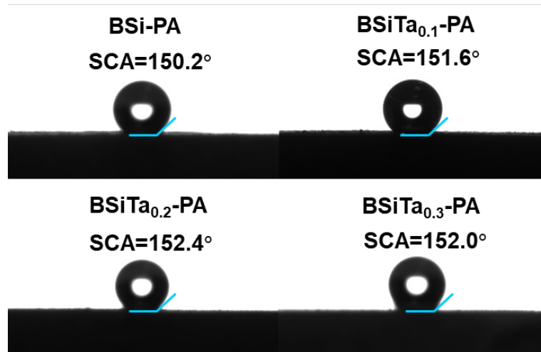
Fig. S5 Static water contact angles of different aerogels
