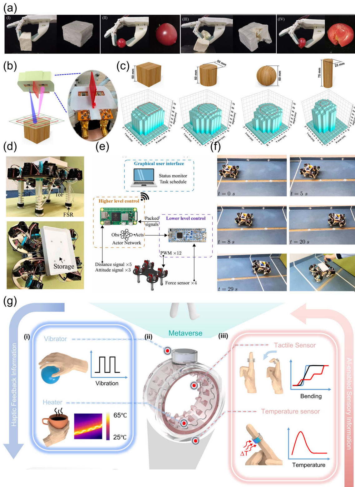
Fig. 13 a Demonstration of grasping tofu and tomato using a manipulator. b Ultrasonic sensor integrated on a soft robot for object profile detection, and c its performance for different topographic profiles. d Photographs of the robot prototype, and e illustration of the control components. f Photographs to verify the robot to conduct transportation tasks. g Schematic diagram for the multimode haptic sensing and feedback
