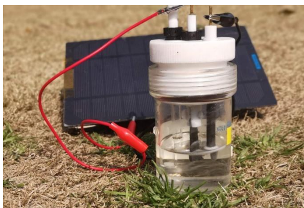
Fig. S4 Solar-energy driven water splitting with EG/(Co, Ni)Se 2 -NC hybrid
