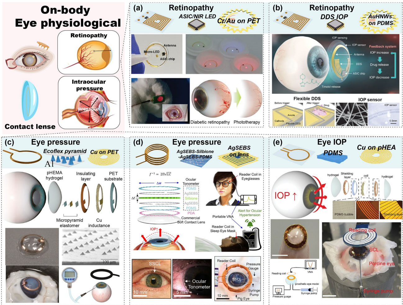
Fig. 12 Wearable device for eye physiological information detection. a Far-red/NiR luminescent contact lens for retinal treatment. Reproduced with permission from Ref. [150]. Copyright © 2022 John Wiley & Sons Inc. b Glaucoma IOP detection-treatment closed-loop contact lens. Reproduced with permission from Ref. [151]. Copyright © 2022 Springer Nature. c Hydrogel smart contact lens for wireless IOP monitoring. Reproduced with permission from Ref. [152]. Copyright © 2022 American Chemical Society. d Commercial contact lens-based IOP monitoring system. Reproduced with permission from Ref. [153]. Copyright © 2022 Springer Nature. e Circle-shaped passive wireless IOP contact lens. Reproduced with permission from Ref. [154]. Copyright © 2024 John Wiley & Sons Inc
